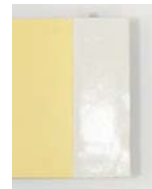
Remove 5/8" of tape from each end of breadboard.
